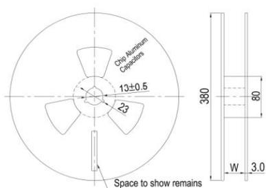
Fig. 2-2 Reel Polarity
