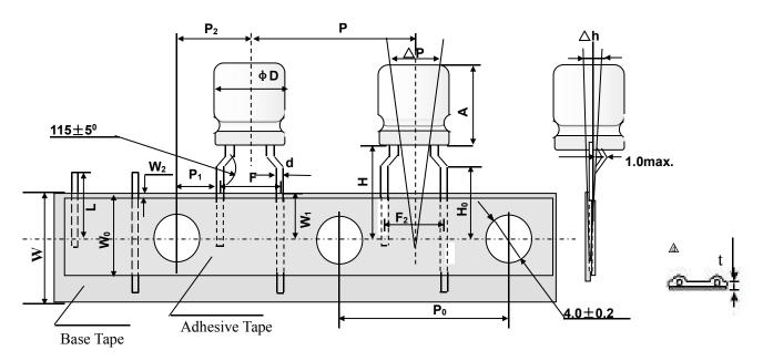
Taping dimension Unit: mm
