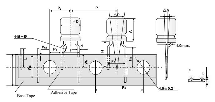
Taping dimension Unit: mm
