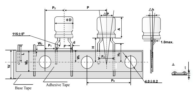
Taping dimension Unit: mm
