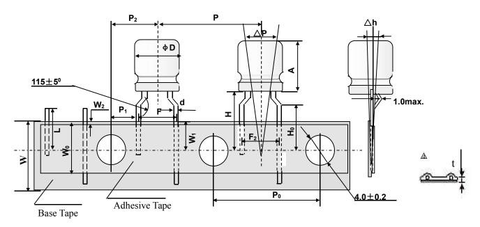
Taping dimension Unit: mm
