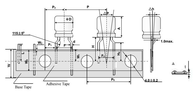
Taping dimension Unit: mm
