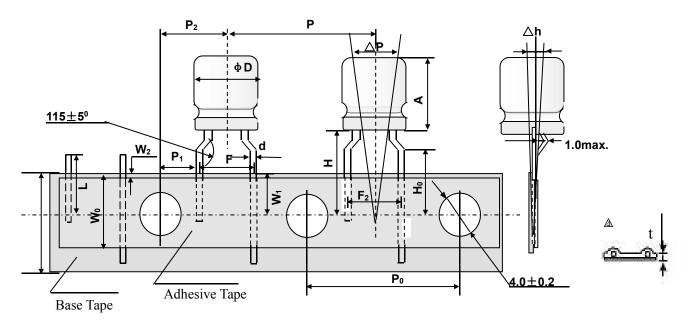
Taping dimension Unit: mm
