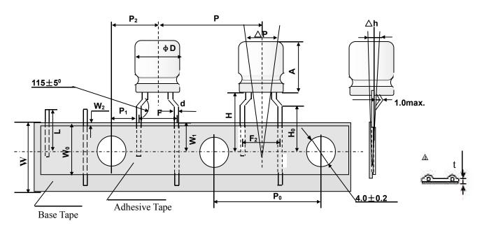
Taping dimension Unit: mm
