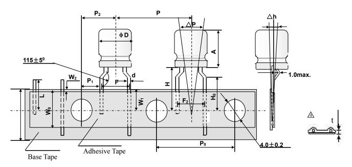
Taping dimension Unit: mm
