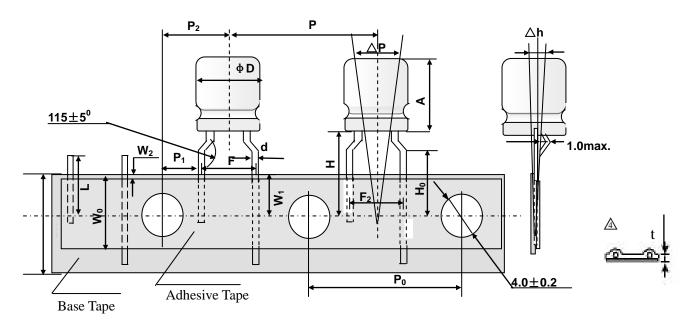
Taping dimension Unit: mm
