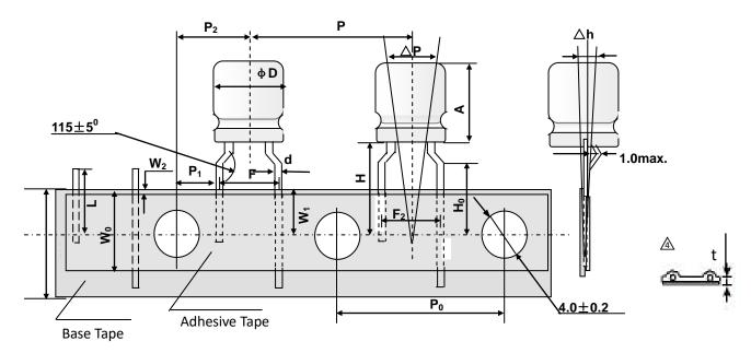
Taping dimension Unit: mm
